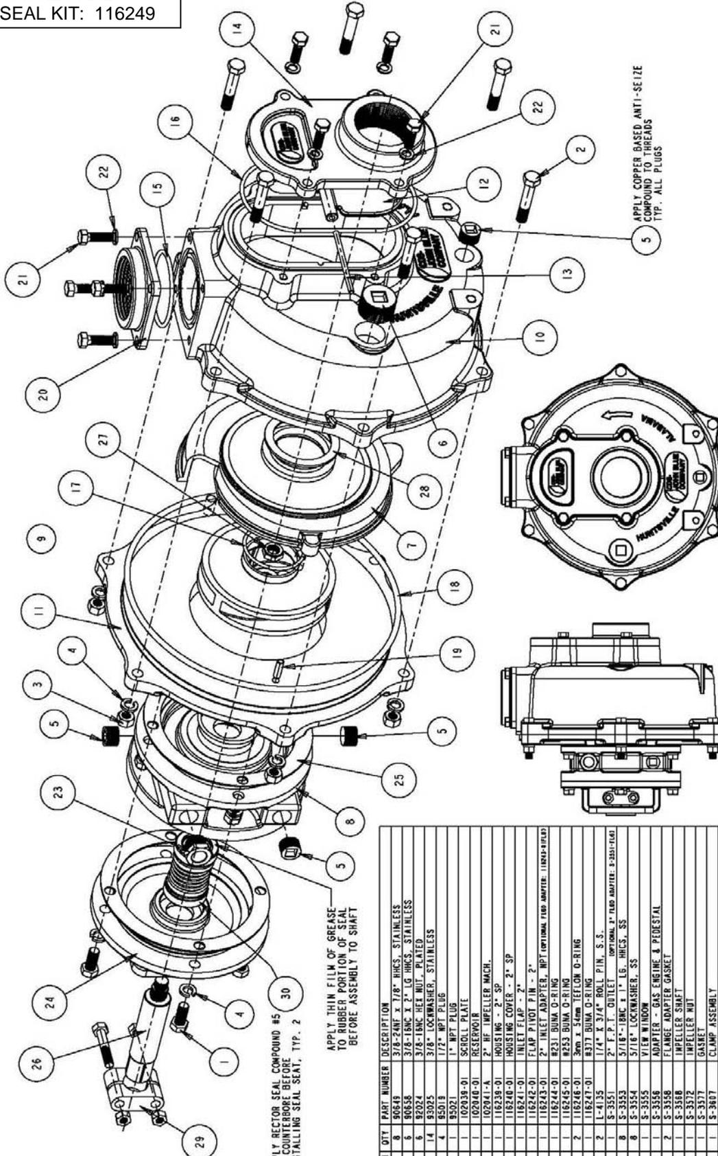
APPLY COPPER BASED ANTI-SEIZE COMPOUND TO THREADS TYP. ALL PLUGS
