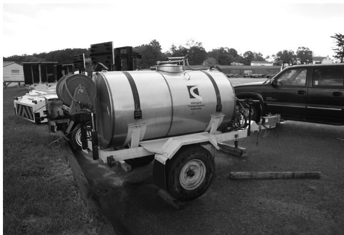
500 gallon stainless steel tank with high pressure diaphragm system
