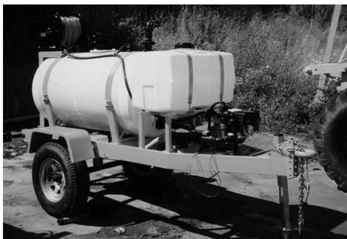
200 gallon sprayer with high capacity centrifugal pump and rinse system
