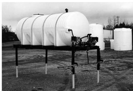
50 gallon pull unit with 15' boom Ideal for parking lots, college campuses and sidewalk treatment
