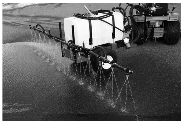
50 gallon pull unit with 15' boom Ideal for parking lots, college campuses and sidewalk treatment
