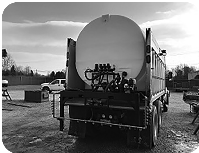
3400 GALLON SUPER NURSE TANK BOOM WIDTH COVERS 3 LANES
