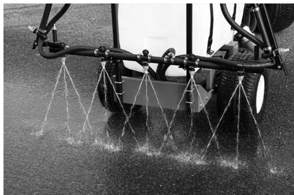
Shown with center boom only for sidewalk work
