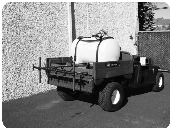
65 GALLON LEG TANK BOOM COVERS 5 FT
