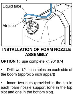
Place each foam support on top of the drilled hole.
