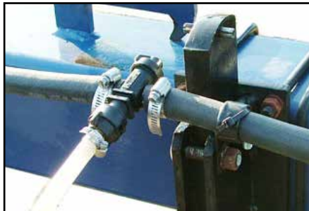
CP2488 diaphragm check valve double shank
