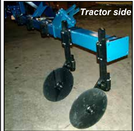
Primary and secondary wings coulters mounting
