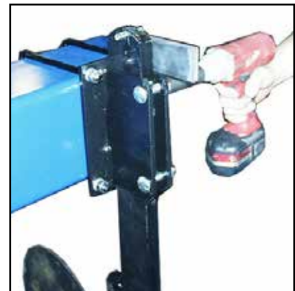
Primary and secondary wings coulters mounting
