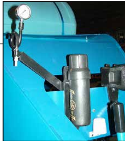
Manual holder mounted with gauge holder mount. Gauge holder part of manifold package.
